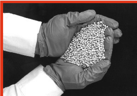
Not Bunny Chow: These pea-size pellets are RVS-1—the regenerable desulfurization sorbent that represents a breakthrough in state-of-the-art coal and fuel gas cleaning.
