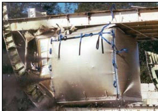
Telair HULD during blast test of aircraft section
