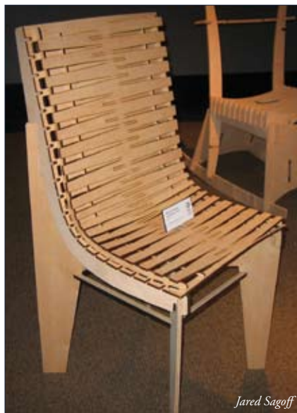
This chair, built by students at the Barcelona Fab Lab, was created from a single 4-by-8 foot piece of plywood manipulated using the Fab Lab technology.
