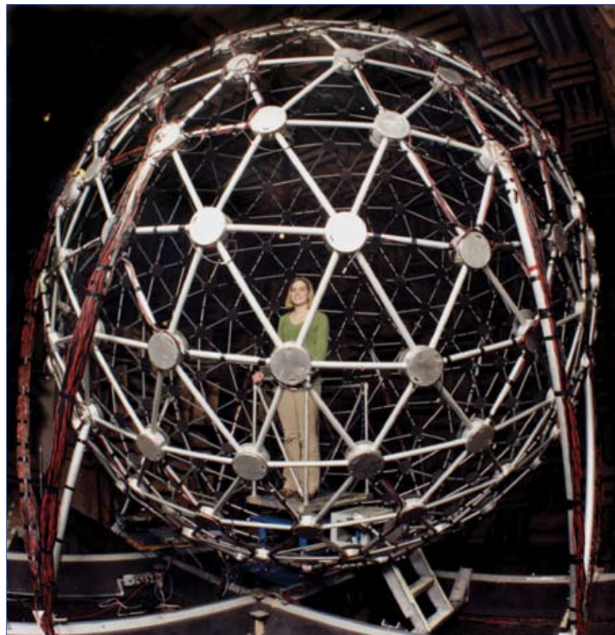
The Auditory Localization Facility (ALF) at the Air Force Research Laboratory's Human Effectiveness Directorate enables research in binaural and spatial hearing, measurement of head-related transfer functions, and development of 3-D audio systems. ALF is a 4.26-meter-diameter geodesic sphere inside an anechoic chamber. The sphere contains 277 loudspeakers and can present 16 sounds simultaneously from selected or all locations, simulating complex real-world auditory environments.
