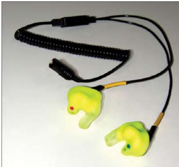
This is the ruggedized version of the ACCES system, shown complete with earplugs and associated cables/electronics.
