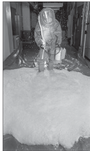
A nonhazardous decontaminating foam developed at Sandia begins neutralizing both chemical and biological agents in minutes.
