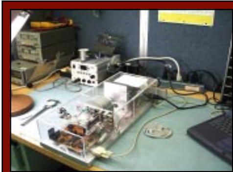
Developed from the standard for the electronic book file, the Braille Reader is low in cost and is accessible in assisting visually impaired individuals to read web pages and e-book files. Pictured is the NIST rotating wheel Braille display.
