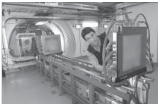
In NSRL's target room, Adam Rusek checks the cabling of one of the four ion chambers used for beam imaging.
