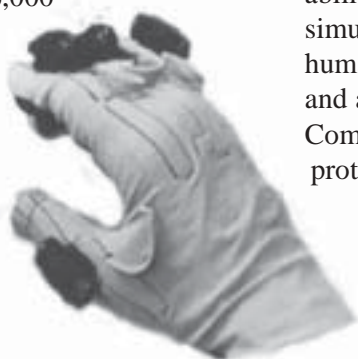
RDHFL's cyber glove system provides tactile feedback and high-accuracy joint measurements of the human hand that can be used to interact with virtual environments.
