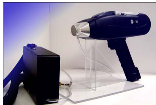
The Vacuum Enhanced X-ray Fluorescent Scanner
