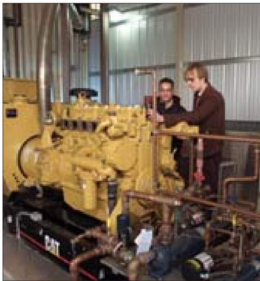
LLNL engineers Francisco Espinosa-Loza and Daniel Flowers work on the stationary homogeneous charge compression ignition engine.
