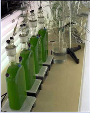
System for photobiological algal hydrogen production.
