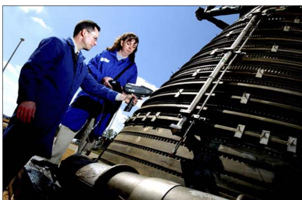
Richard Booth, left, MSFC Engineering Directorate, and Wanda Hudson, ATK Thiokol, use the scanner to analyze materials in an F-1 engine.
