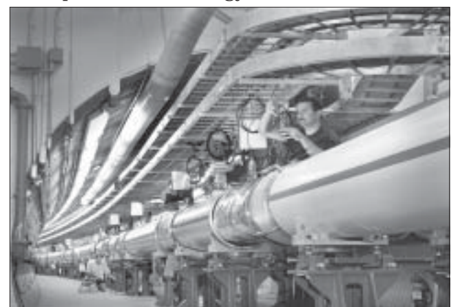
A view of the superconducting magnets at BNL's Relativistic Heavy Ion Collider. As gold particles zip along the collider's 2.4-mile-long tunnel at nearly the speed of light, 1,740 of these magnets guide and focus the particle beams.
