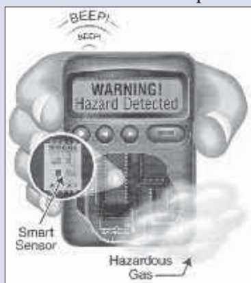
The Smart Sensor Developer Kit consists of a dime-sized sensing element and onboard signal processing, measurement, and analysis capabilities in a system smaller than a pocket pager.
