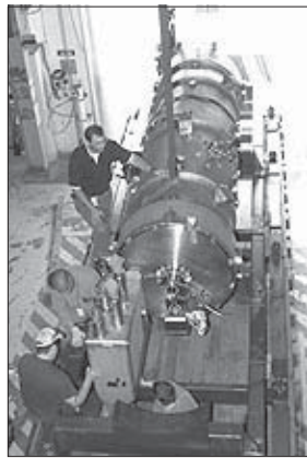
Researchers work on a cryomodule for the DOE's new Spallation Neutron Source facility.
