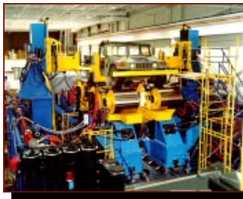
The new roadway simulator at the Aberdeen Test Center.
