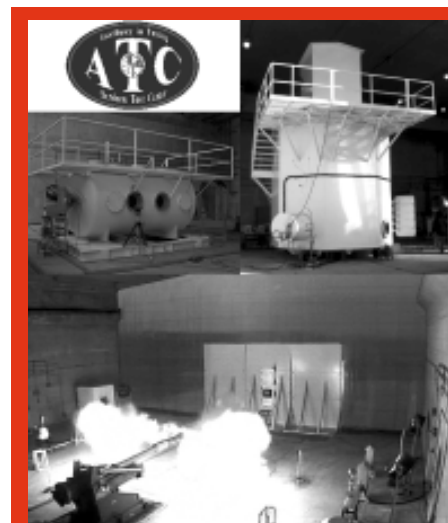
Clockwise I to r: ATC's emission characterization chamber, ATC's large octagon test chamber (LOTC), Bottom: Emissions test in ATC's modified large caliber firing barricade.
