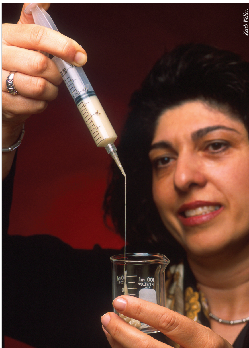
A soy-based polymer slurry being tested by chemist Sevim Erhan can be used with or without molds to make small toys or manufacturing parts.
