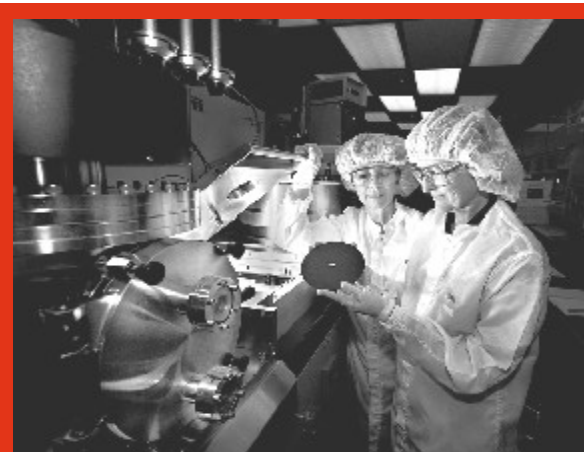
Sandia researchers Carol Ashby (foreground) and Carolyn Matzke prepare to put a wafer sample into a high-density plasma chamber used to deposit thin films on wafers. At the center of the wafer is a thumbnail-sized chip laden with the makings of tiny fluidic canals. (Photo by Randy Montoya)
