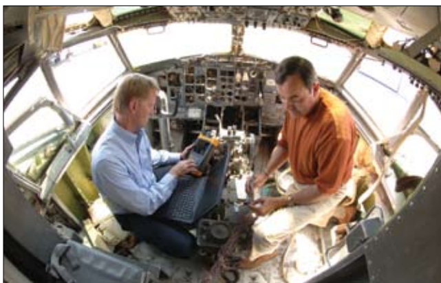
Larry Schneider (left) and Mike Dinallo use the PASD diagnostic on a cockpit wiring bundle in a retired Boeing 737 at a Sandia FAA test center.
