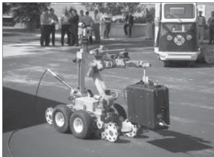
The Kansas City Police Department's robot carries the PIRATE device during a demonstration at the Kansas City Plant. A scenario was created for the demonstration where an individual was handcuffed to the steering wheel of a car and a suspicious package with a substance seeping from it was under the vehicle.
