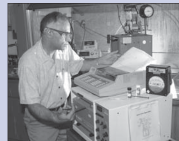
Researcher Devinder Mahajan uses a gas chromatograph to analyze carbon monoxide levels in hydrogen purified using his patented process.
