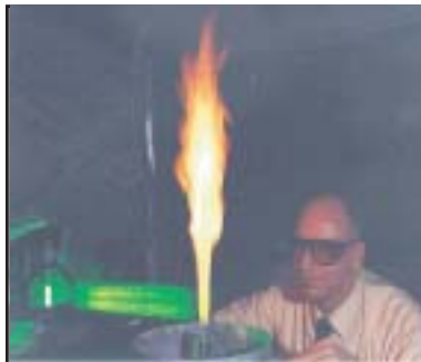
Dr. William Roquemore examines a jet diffusion flame with a laser sheet lighting technique invented by his team at AFRL's Propulsion Directorate.
