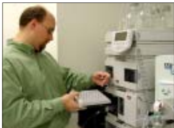
Using liquid chromatography and mass spectrometry instrumentation, Pacific Northwest National Laboratory scientists identified and characterized nearly twice as many proteins in blood serum than previously noted.
