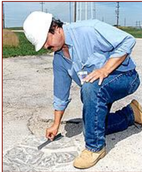
Argonne's Pat O'Malley measures a circular Ceramicrete patch.
