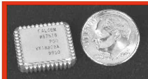
Picosecond Timing: An integrated circuit developed at Sandia National Labs can make picosecond timing measurements without leading-edge circuit speed or high-speed clock.
