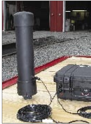
The GPS-enabled cell phone in weather-resistant pod and battery pack that connects to locomotive power supply.
