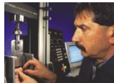
Animal Physiologist Mohammad Koochmaraie uses an electronic testing machine to measure the tenderness of a sample sheared from a cooked steak.
