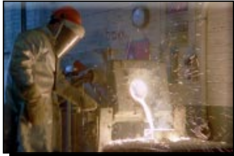
Castings are developed by modifying the evaporative pattern casting (EPC) process for aluminum casting and applying it to steel.
