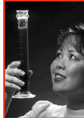
Super Glue: Research associate Mila Hojilla-Evangelista prepares a sample of soy-based plywood adhesive to test its foaming ability. The glue is designed to be applied by foam extrusion.
