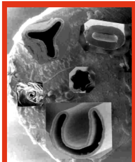
Thin is in: Several microtubes are superimposed over a human hair with a width of 100 microns.
