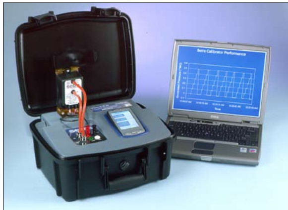
Setra's MicroCal™ Low Pressure Calibrator incorporates NASA technology.
