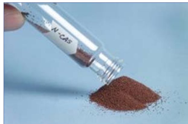
INL researchers developed a long-lasting, high-capacity nano-composite polymer particle engineered to remove arsenic concentrations from water, rendering it safe to drink and compliant with U.S. and world standards.
