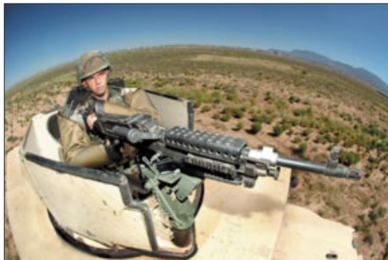
ARMS PROTECTION —Airman Garrett Martin demonstrates the SNL gauntlet atop a Humvee at Albuquerque's Kirtland Air Force Base. The gauntlet can help save the arms and lives of military personnel riding atop military vehicles during combat operations.
