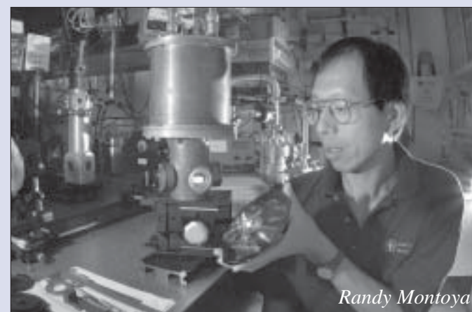
A tungsten photonic lattice glows in a vacuum chamber as SNL researcher Shawn Lin inspects an iridescent disk that contains approximately 1,000 tungsten photonic lattices. Most emissions from these filaments are in the near-infrared range, and may improve efficiencies of heat-driven engines like hybrid electric automobiles.
