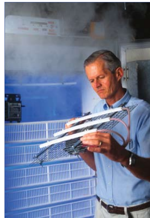
Agricultural engineer Bailey Mitchell demonstrates an electrostatic air cleaning system. The hatching cabinet used here is a small version of ones used commercially for hatching chicks.
