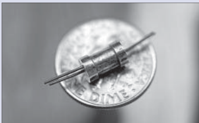
The Milli-Watt System Fuel Processor converts methanol into hydrogen and carbon dioxide and can be used in very small fuel cells to generate electric power. It is the smallest integrated catalytic fuel reformer in the world.
