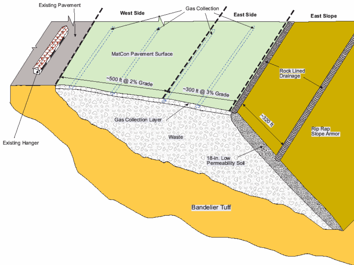
Figure 4. Alternative 2, MatCon™ Cover and Rock Armor.
