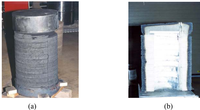
Figure 6. Outside surface of the Celotex ring segments after the HAC thermal test of a Model 9975 packaging, (a), and cross-sectional view of the Celotex showing the charred outer layer, (b).
