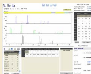
Figure 2. FSS-i3 ® spikeogram of Profiler Plus ® 1:2 mixture ratio replicate 1a and the i-STRem program interface.
