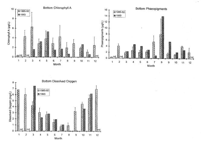
FIGURE 3.19. Bottom-water quality for station C6\* (composite data for Stations C6A, C6B, and C6) for 1985–92 average conditions ( $\pm$  s.e.) compared with 1993. NOTE: *n* for average condition ranges 10–30 in March–October and 2–6 in November–February; *n* for 1993 is 1 or 2. (From Rabalais et al. 1998.)
