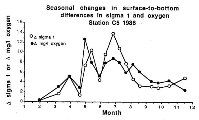
FIGURE 4.4. Differences in surface- to bottom-water values for sigma t and dissolved oxygen concentration by month for station C5 during 1986. (From Rabalais et al. 1991.)
