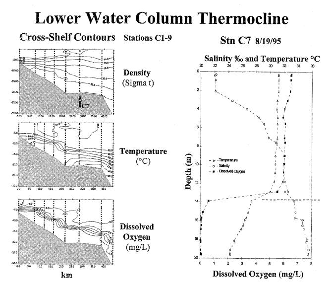
FIGURE 4.7. Cross-shelf contours of density, salinity, and dissolved oxygen for 19 August 1995 with vertical profiles of salinity, temperature, and dissolved oxygen for station C7. (Rabalais et al. unpublished data.)
