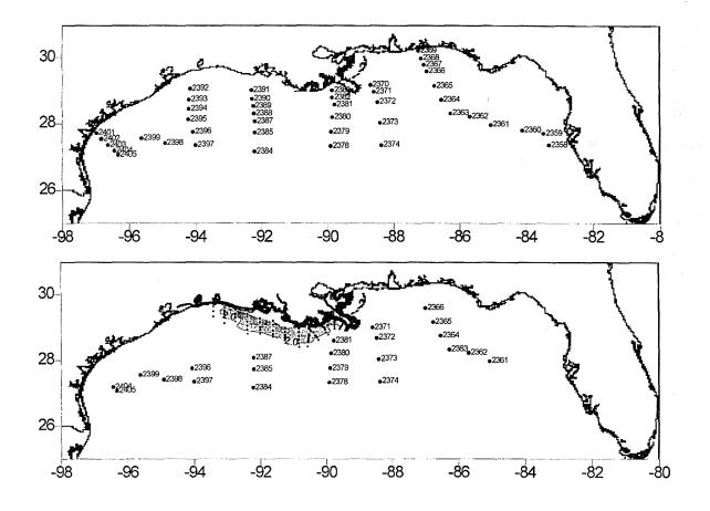
FIGURE 7.1. Upper panel: Stations from the 1935 M/V Atlantis surveys of the Gulf of Mexico north of 27°N. Bottom panel: M/V Atlantis stations with mid-water dissolved oxygen concentrations less than 3 cm<sup>3</sup>/l (N.T.P.) (= 4.3 mg/l), compared to the hypoxic zone of July 1996. (M/V Atlantis data from Conseil Permanent International pour l'Exploration de la Mer (1936); July 1996 data from Rabalais et al. unpublished data.)
