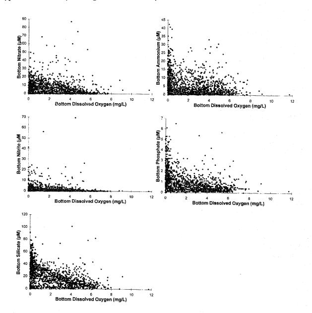
FIGURE 6.17. Comparison of bottom-water dissolved oxygen concentration and bottomwater dissolved inorganic nutrient concentrations for all stations and all depths for May-September 1985-96. (From Rabalais and Turner unpublished data.)
