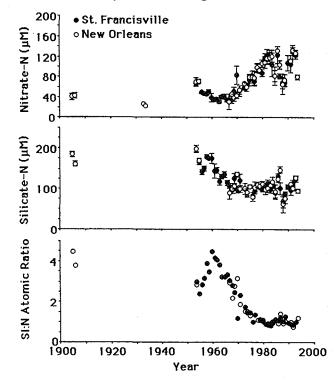
**FIGURE 5.4.** Changes in nitrate and silicate and the Si:N ratio from 1905 through 1994. NOTE:  $\bullet$  for St. Francisville,  $\bigcirc$  for New Orleans; bars are  $\pm$  s.e. of the average of monthly means. (Modified from Turner and Rabalais 1991 in Rabalais et al. 1996.)
