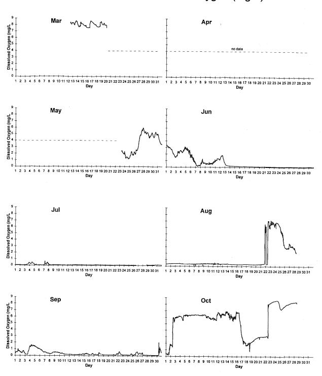
Station C6B 1996 Bottom Oxygen (mg/L)
