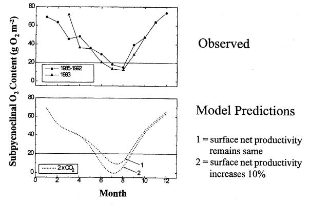
FIGURE 9.1. Seasonal changes in the oxygen content of the lower water column during 1985–92 and 1993 (top panel), and model predictions for a doubled  $CO_2$  climate (bottom panel). NOTE: Two model predictions for total oxygen content of the lower water column are shown: (1) integrated net production remains the same as during 1985–92; and (2) the net production value for the May-August period is increased by 35%. (From Justicet al. 1996.)
