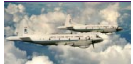
NOAA's WP-3D Orion aircraft were equipped with Stepped Frequency Microwave Radiometers during the 2004 hurricane season to obtain observations of ocean surface winds.
