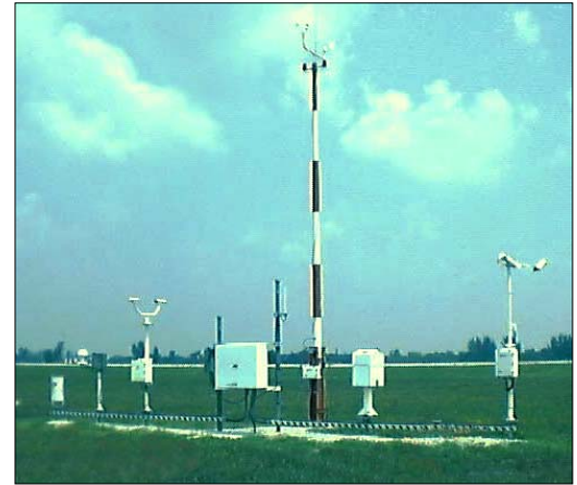
Photograph of a typical automated surface observation weather station (Opa Locka, Florida) used for documenting wind exposure.
