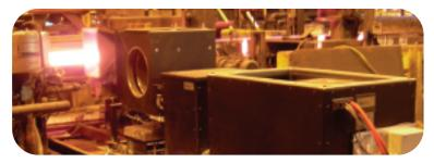
The HotEye™ system uses imaging technology to inspect newly forged metals while withstanding their intense heat. It can cut waste of forged metal product by 90 percent and reduce burn injuries, with a resulting savings to U.S. industry in the billions.
