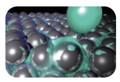
Three-dimensional printing process technologies created by Extrude Hone Corporation could enable low-cost manufacture of Styrofoam patterns for complex engine components from a parts-design database. In this conceptual image, print heads selectively deposit micro droplets of binding solution with extreme precision only on the powder to be printed, bonding each layer until all cross-sections have been built.
