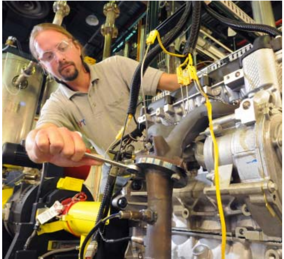
Argonne mechanical engineer Thomas Wallner adjusts Argonne’s “omnivorous engine,” an automobile engine that Wallner and his colleagues have tailored to efficiently run on blends of gasoline, ethanol and butanol.
