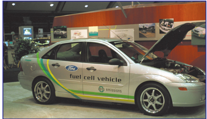
Fuel Cell zero emissions vehicle combines hydrogen fuel with oxygen from the air to create electricity for power.
