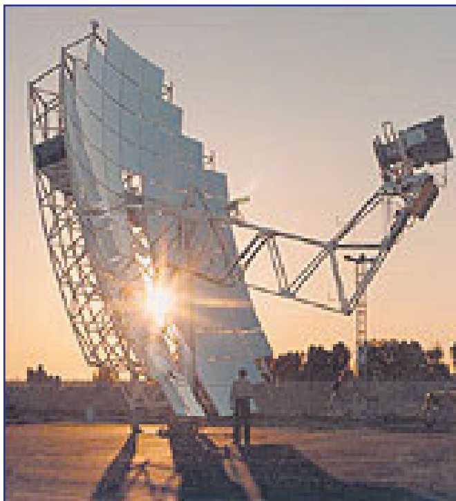
This solar dish-engine system is an electric generator that “burns” sunlight instead of gas or coal to produce electricity. The dish, a concentrator, is the primary solar component of the system, collecting the energy coming directly from the sun and concentrating it on a small area. A thermal receiver absorbs the concentrated beam of solar energy, converts it to heat, and transfers the heat to the engine/generator.
