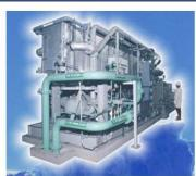
Air Products and Chemicals' Closed-Cycle Nitrogen Refrigeration (CCNR) compresses, cools, and condenses liquid natural gas that would otherwise be lost to the atmosphere during transport.
