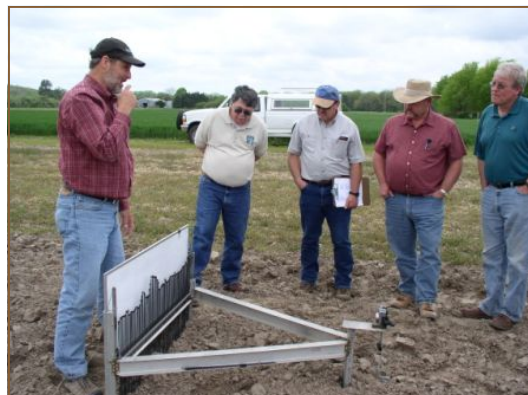
Tatarko (L) explains the pin method for determining field roughness to workshop participants.
