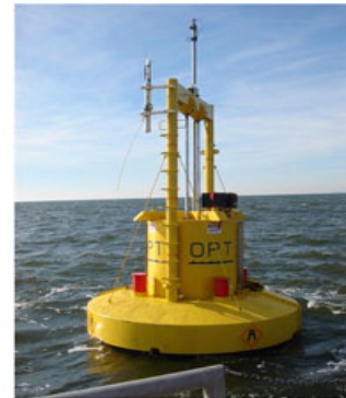
Point Absorber (OPT Power Buoy)
