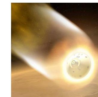
The capsule will perform a direct entry at Earth. After entry the capsule will free-fall until approximately 3 kilometers (1.8 miles), at which point the parachute deployment sequence will initiate. Elapsed time from entry to parachute deployment will be approximately 10 minutes.
