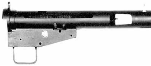
STEN MK II submachinegun receiver
