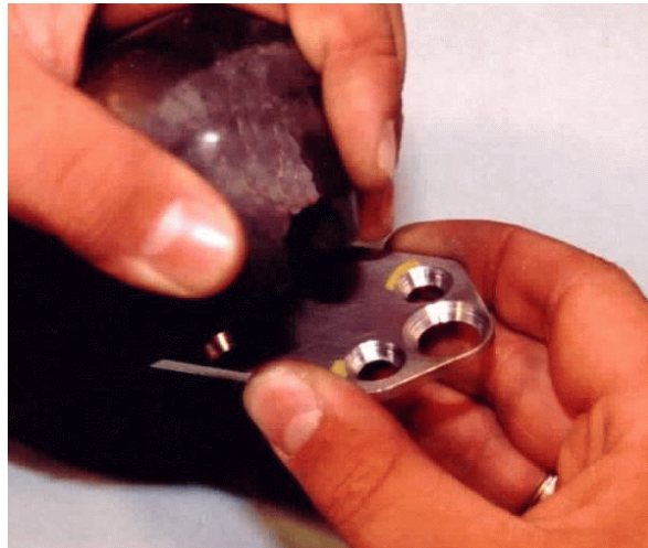
Figure 13.23- Insert the Ankle / Achilles Mounting Plate
