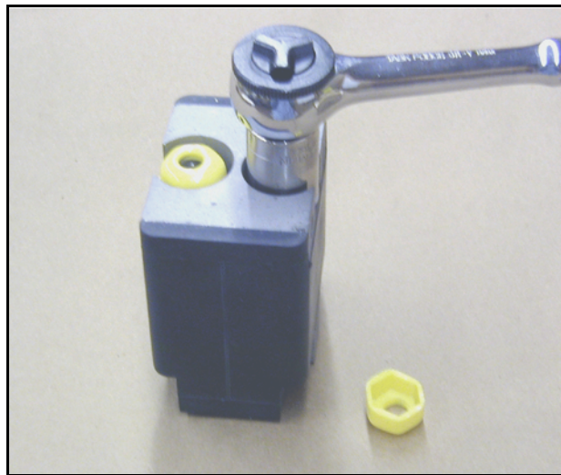
Figure 6.19- Tightening the Flex Joint Cables
