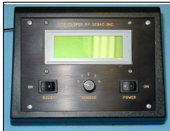
Figure 15.11- Front-view of tilt sensor readout display
