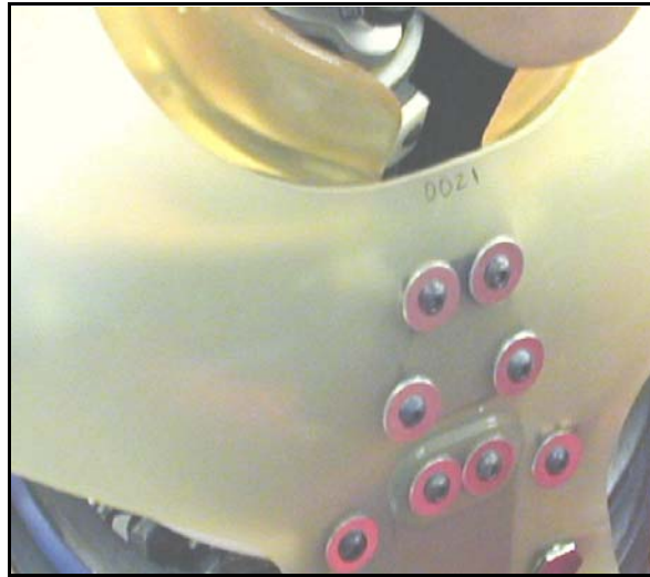
Figure 7.16- Attach bib to Upper Sternal Plate
