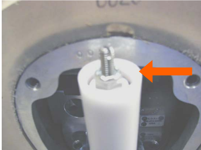
Figure 3.10- Rear Spring Adjustment Locknut Location
