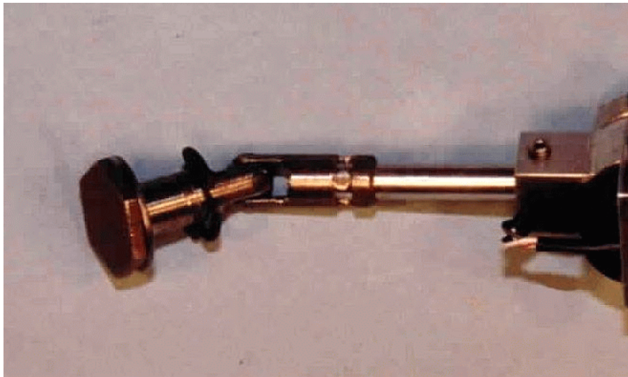
Figure 16.12- U-Joint centered in its range of motion
