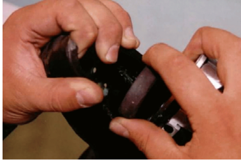
Figure 13.27- Insert rubber heel pad
