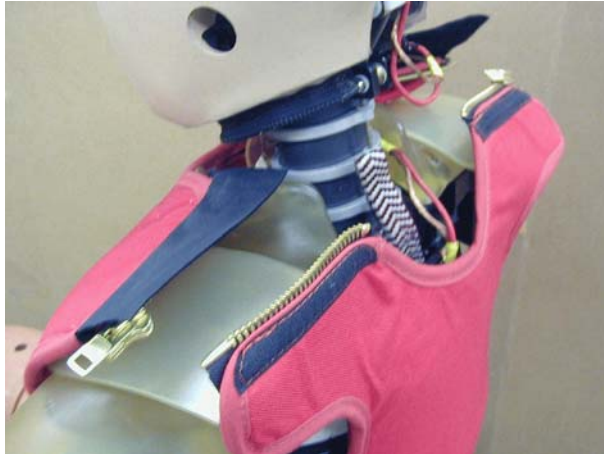
Figure 14.4- Jacket assembled onto thorax
