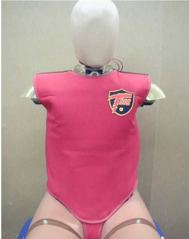
Figure 14.9- Properly installed Jacket assembly (front).
