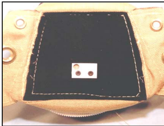
Figure 9.12- String potentiometer / accelerometer mounting plate
