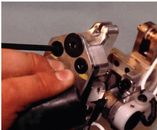
Figure 13.26- Attach the Achilles Cable Mount
