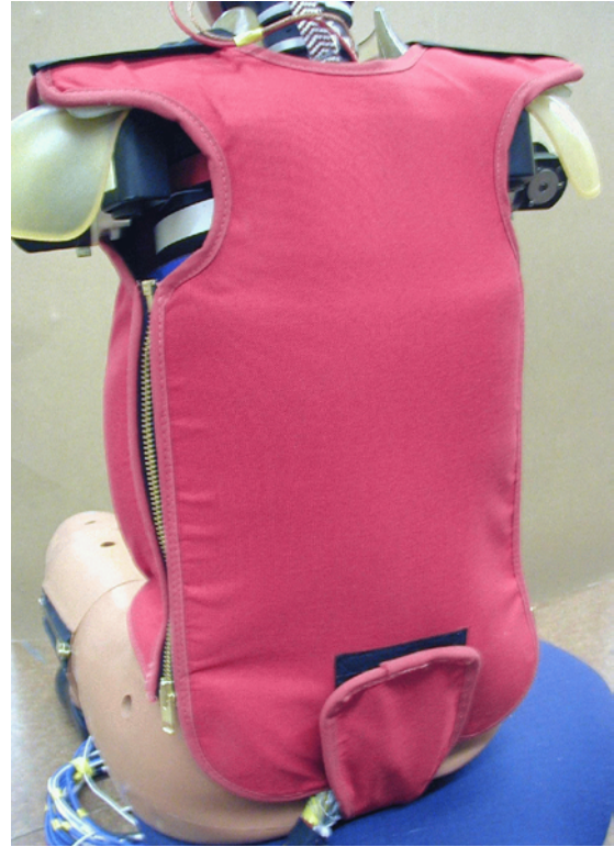
Figure 14.10- Properly installed Jacket assembly (rear).
