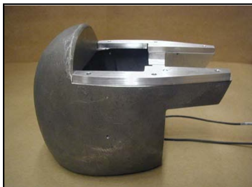
Figure 4.3- Face Plate Spacers/Head Skull Assembly
