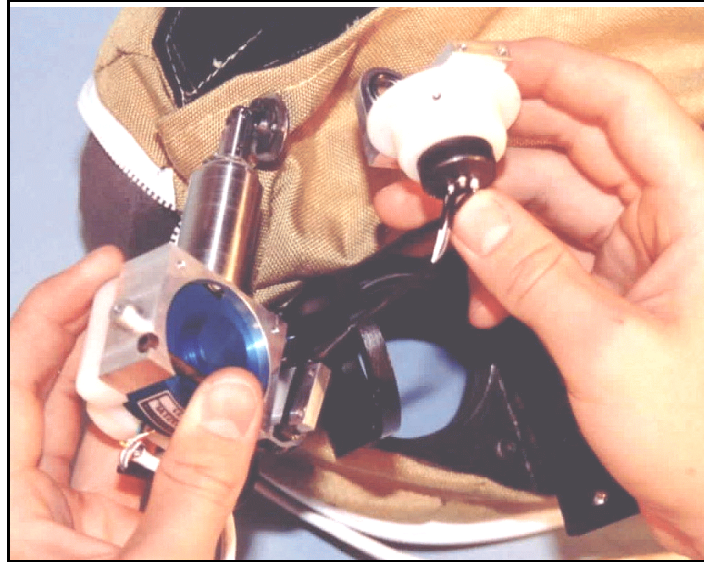
Figure 10.9- Potentiometer wire routing through slot in rear of bracket
