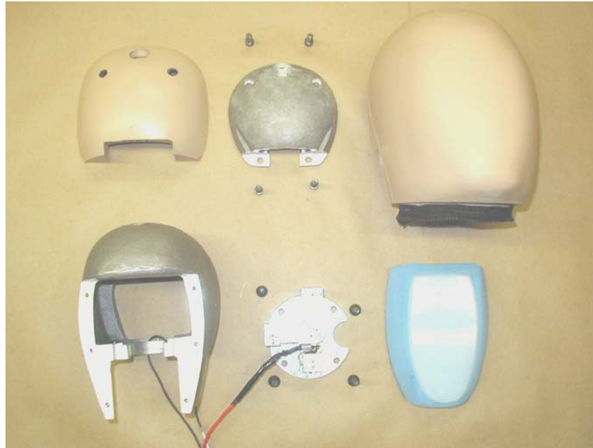
Figure 3.2- Head Exploded Assembly
