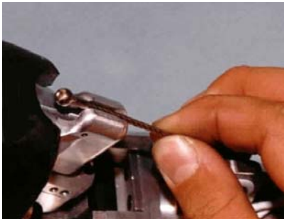
Figure 13.28- Slide cable ball into slot
