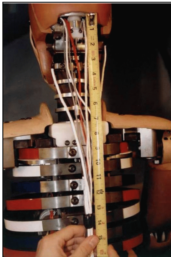
Figure 7.5- Measuring the wire bundle
