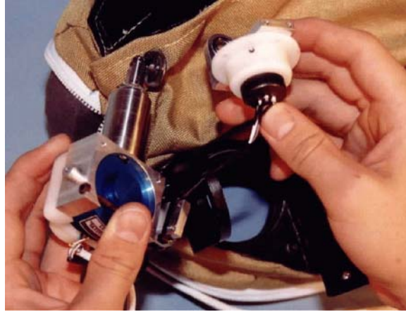
Figure 17.6- Route potentiometer wiring through slot in plate
