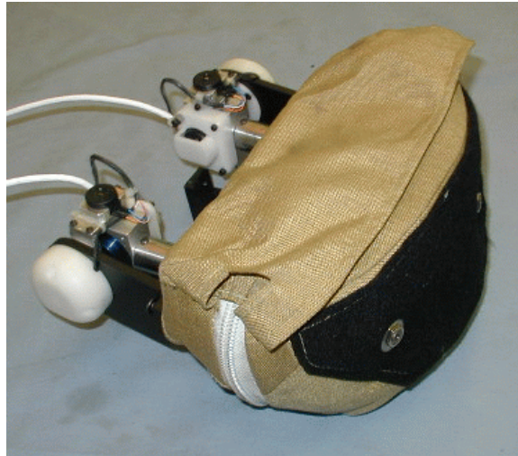
Figure 17.17- Complete DGSP assemblies installed in the Lower Abdomen
