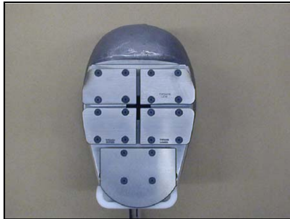
Figure 4.6- Load Cell Plates attached to Load Cells
