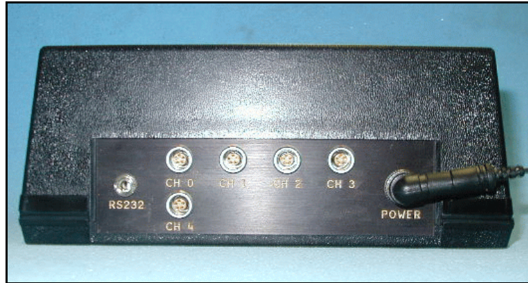
Figure 15.10- Connecting tilt sensors to the display
