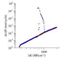
Effect of hydrogen on fatigue rate
