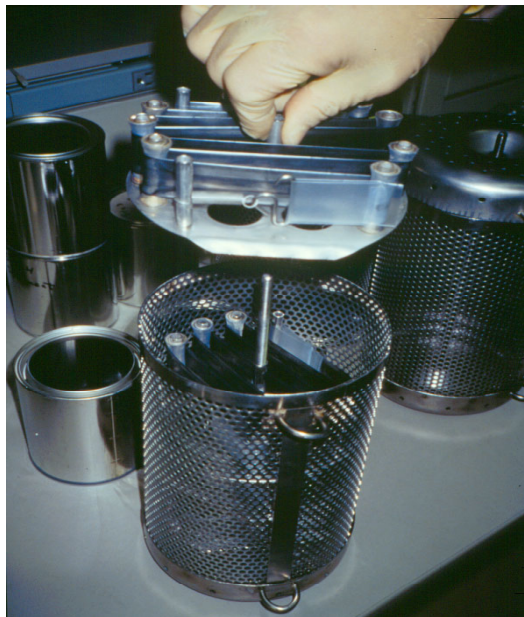
Figure 2. A commercially available stainless steel deployment apparatus, which has a capacity of 5 Standard SPMDs. Each SPMD is placed on a separate rack and the five racks are held in place by a threaded center pin as shown in the picture.
