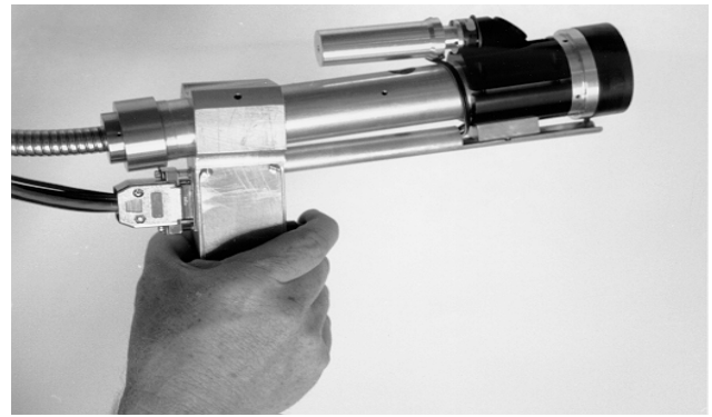
Figure 1. Shown above is the prototype handheld laser leak detector. The armored fiber optic cable exits from the rear of the laser barrel to the left of the operator's hand. The small metal tube mounted on top of the barrel houses the visible laser guide beam to assist the operator in aiming the detector.
