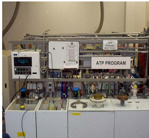
A prototype of a CAM plating workstation incorporates features that could be refined and specified from the CAD system.
