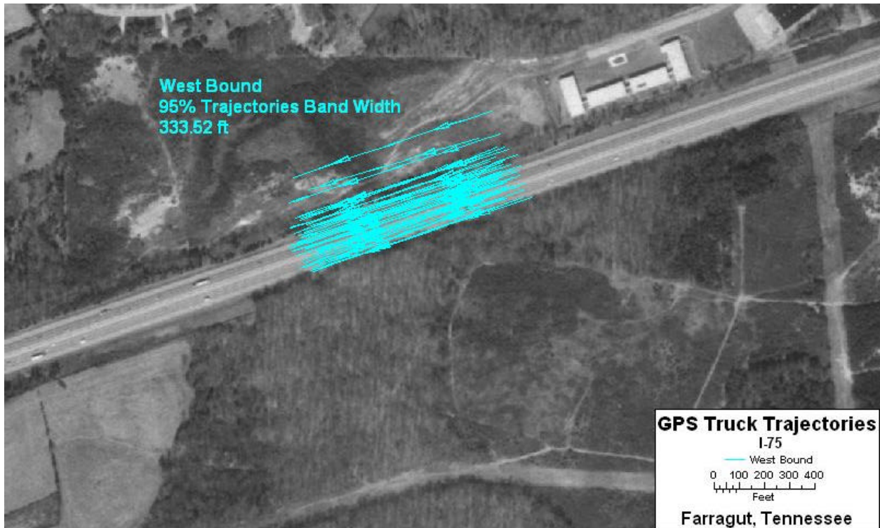
Figure 4.19. West-bound, I-75, pre-May 1, 2001, truck trajectories, measured near Knoxville, Tennessee. Note: band width = 334 feet.
