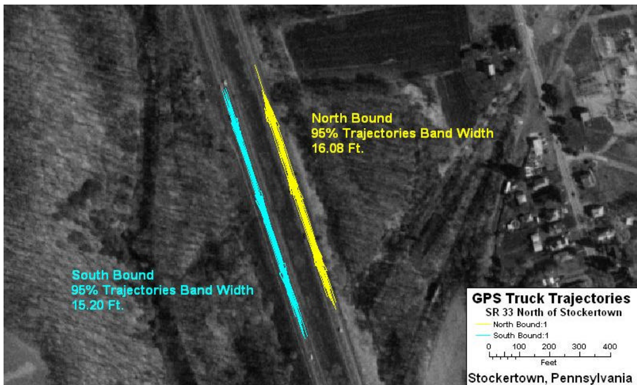
Figure 4.22. North-bound and south-bound, post May 1, 2001, truck trajectories, measured north of Stockertown, Pennsylvania. Note: band widths = 16 feet (north-bound) and 15 feet (south-bound).
