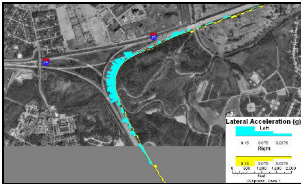
Case 1 – Figure 1. Lateral accelerations measured at the I-24/I-75 junction near Chattanooga, Tennessee.
