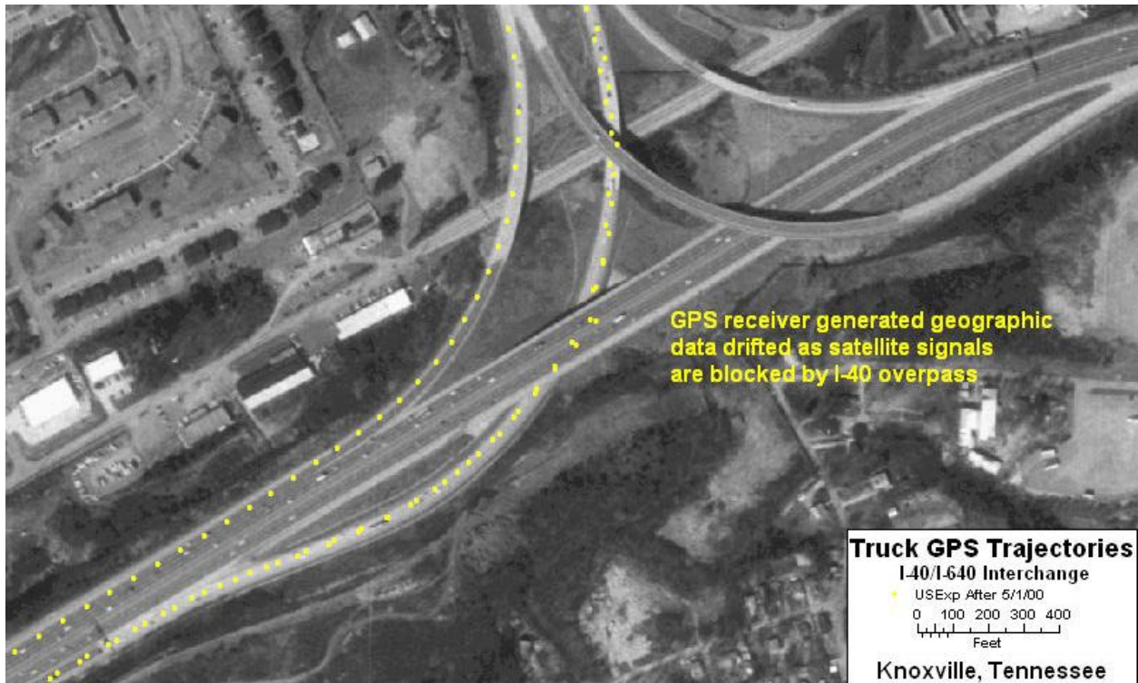
Figure 4.21. North-bound and south-bound, post May 1, 2001, truck trajectories, measured near Knoxville, Tennessee. Note the drift when signals were blocked by the overpass.
