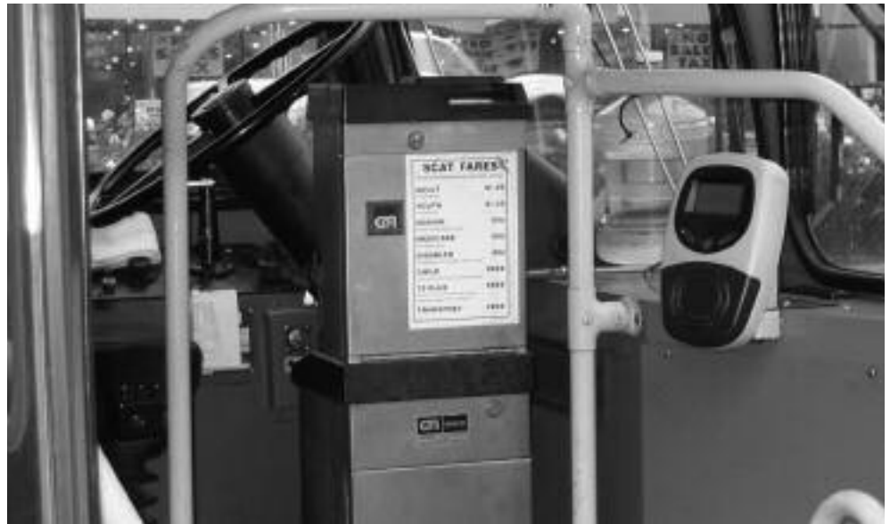
Figure 8 - Smart Card Reader and Fare Box
