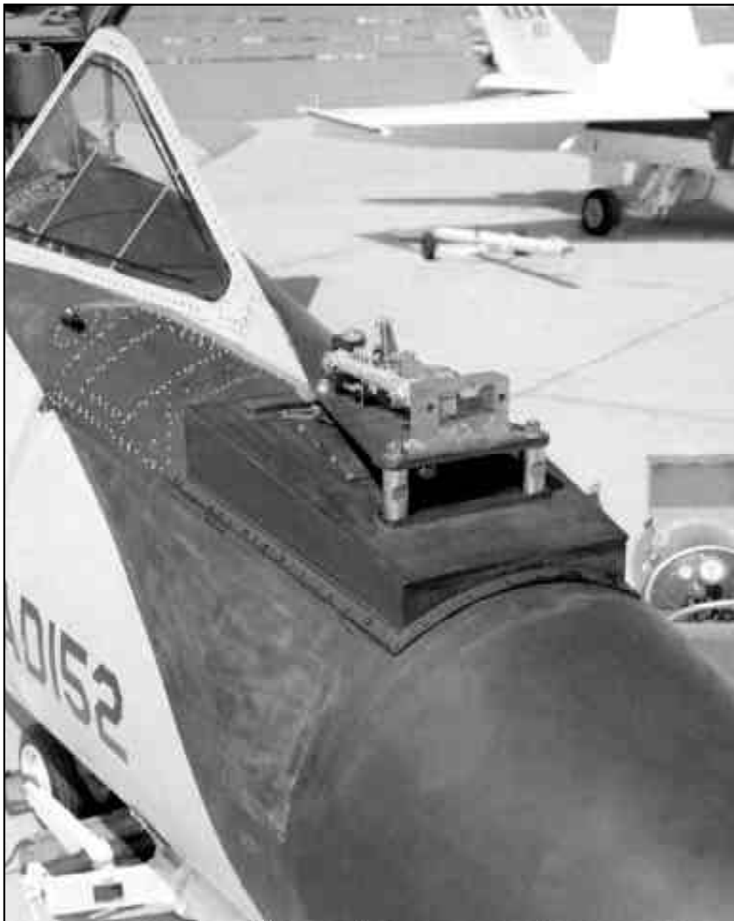
F-106 tow cable attachment and release mechanism for the Eclipse program. (NASA photo EC97 44233-5 by Tony Landis)
