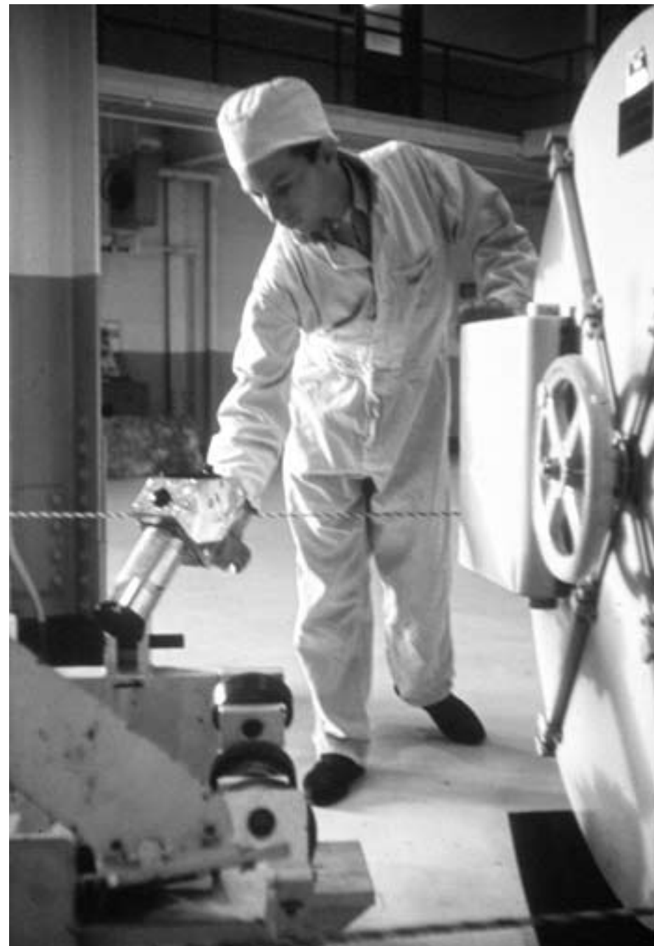
A health physics technician uses a handheld "cutie pie" radiation detector to check equipment for contamination. (NASA C-2003-840)
