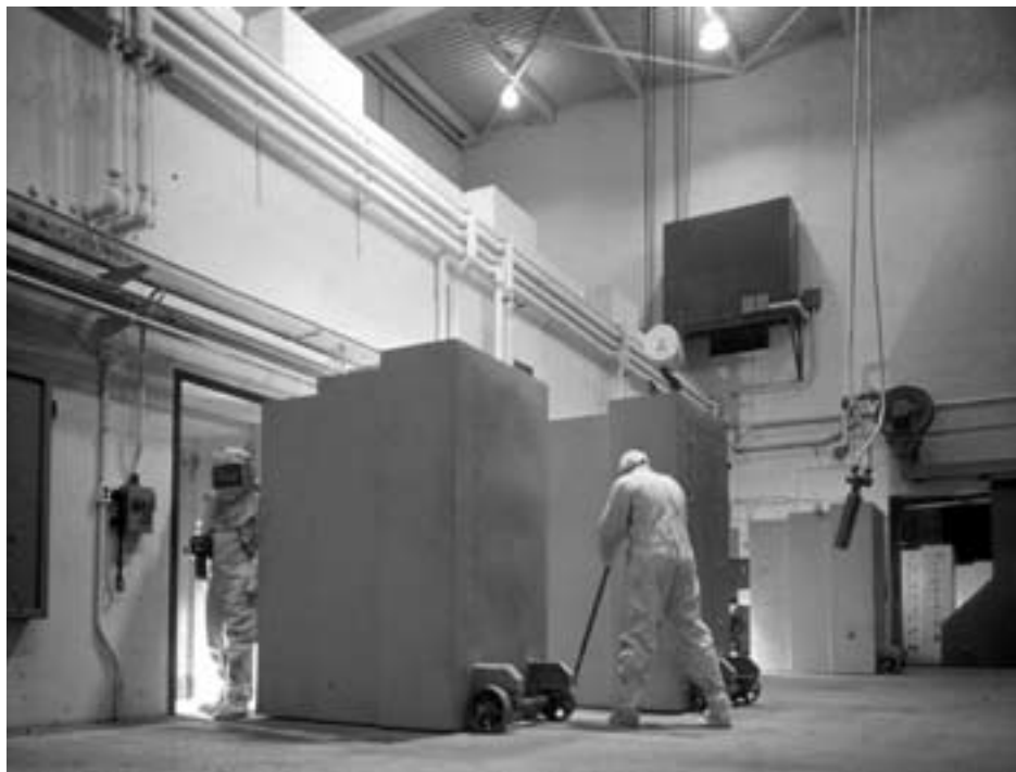
A technician emerges from the rear of the hot laboratory in full protective clothing. Another technician wheels open the massive 63-inch-thick concrete door plug. (NASA CS-22203)
