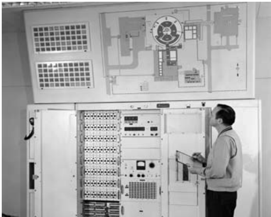
Tom Junod, the Health and Safety Officer, looks at radiation sensing monitoring equipment. The color of the lights indicated the presence or absence of radiation. (NASA 1961_55636)
