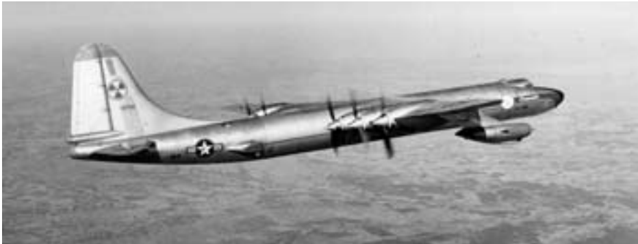
A Convair B-36 bomber converted to operate a nonpropulsive test reactor during flight. It flew 47 times between 1955 and 1957 over Texas and New Mexico. (Department of Energy)
